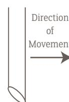
Cut the ends of the tubing at a 45° angle with the long side facing forward into the direction of travel.
