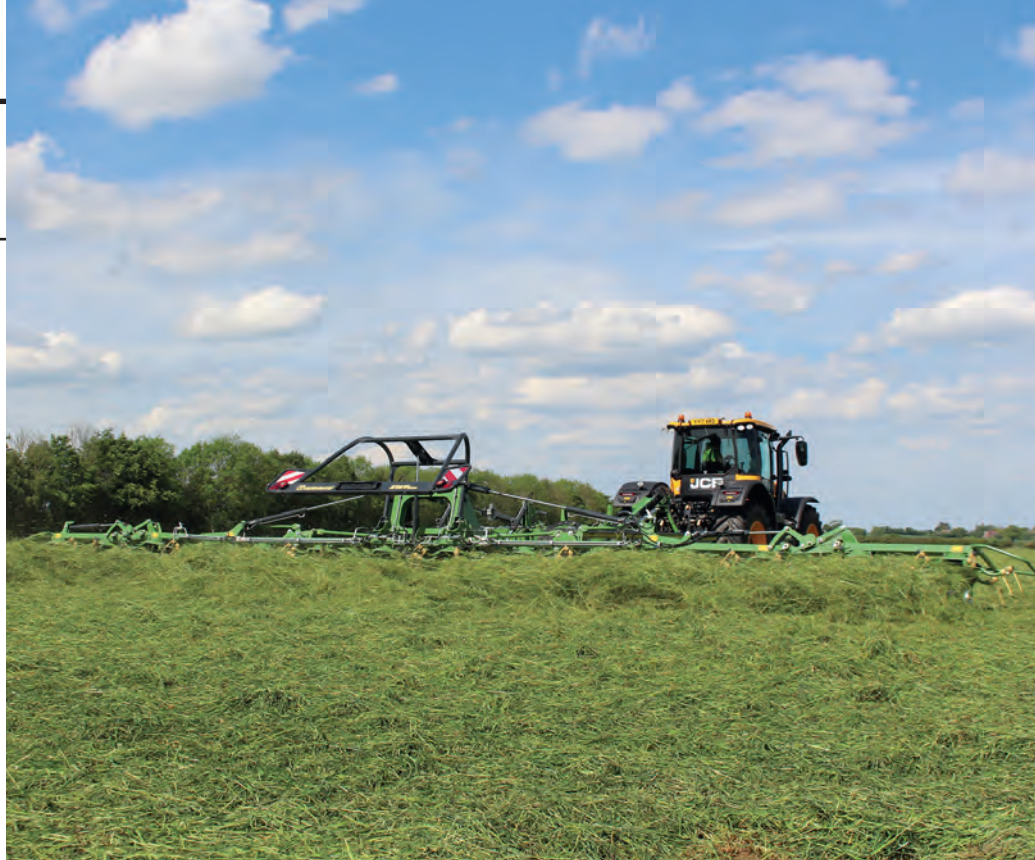
Tedding will help to achieve a rapid wilt and ensure the grass is evenly mixed.
